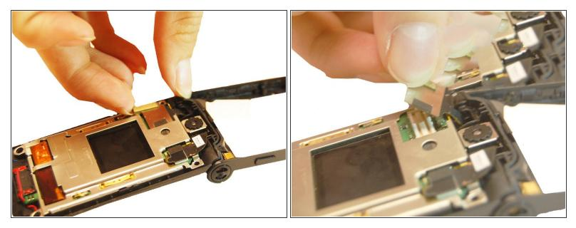
Pull the flex cable connection away from the top of the phone.
