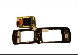
Hold the outer phone casing and pull the LCD screen out.
