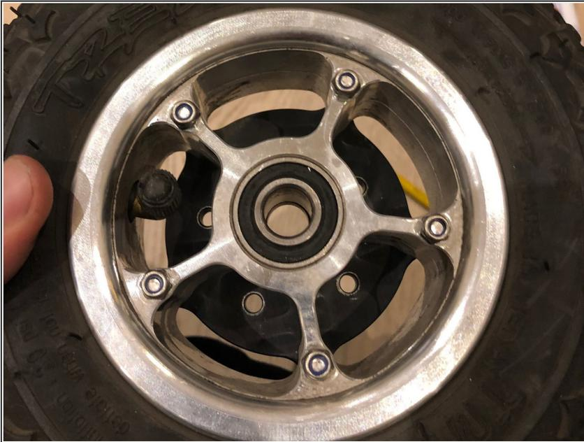
**⚠** Make sure to tighten nuts in star pattern to make sure equal tension on all bolts
