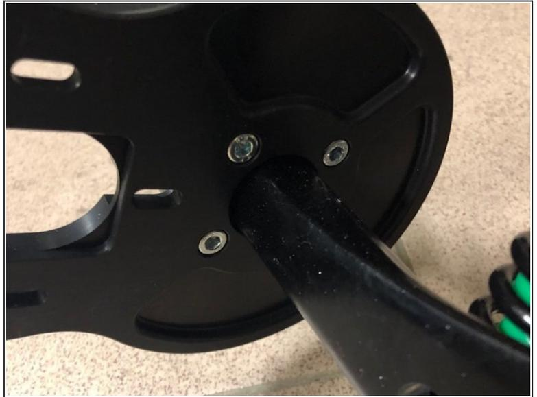
**i** Use Loctite to secure grub screws on mounting hub
