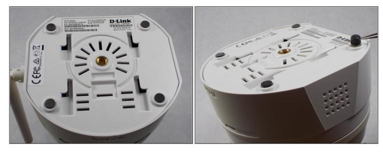
Remove the four rubber feet on the bottom of the camera using your fingers or a pair of tweezers.
