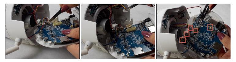
• Disconnect the five quick connections attaching the various cables to the motherboard with your fingers or blunt ended tweezers.
