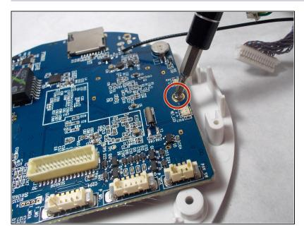
Using a #1 Phillips screwdriver, remove the single 7mm screw holding the motherboard in place.
