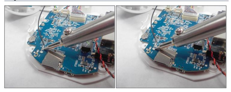
• Using your soldering iron, heat the antenna contacts on the motherboard until the wire releases.
