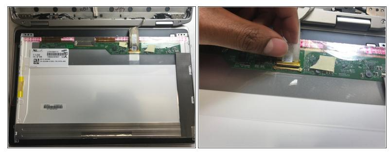
Once all the screws have been removed, lay the screen down on the keyboard and disconnect the LCD cable.
