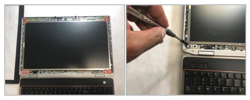
Remove the six 5.75 mm JIS #0 screws that hold the LCD screen to the cover.
