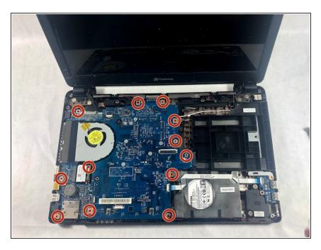
Remove the twelve 3mm screws using the Phillips #00 screwdriver.
