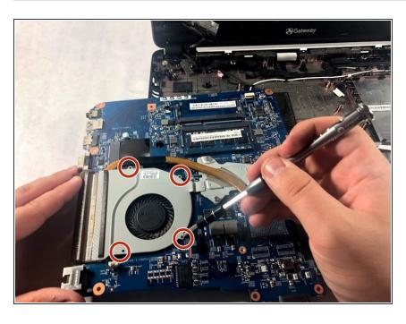
Remove the four 3mm screws attaching the fan to motherboard using the Phillips #00 screwdriver.
