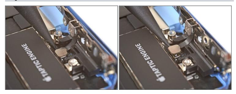
• While holding the bracket out of the way, use the point of a spudger to pry up and disconnect the flex cable underneath.
