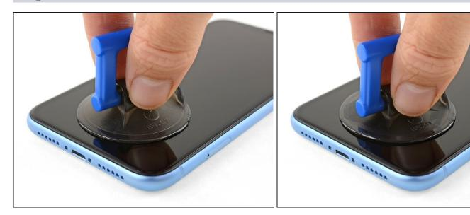
• If you're using a single suction handle, apply it to the bottom edge of the phone, while avoiding the curved portion of the glass.
