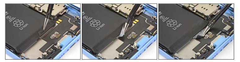
• Peel back the first battery adhesive tab from the bottom right edge of the battery.
