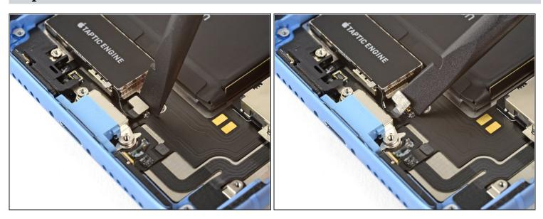
• Use a spudger to disconnect the Taptic Engine flex cable by prying it straight up from its socket.
