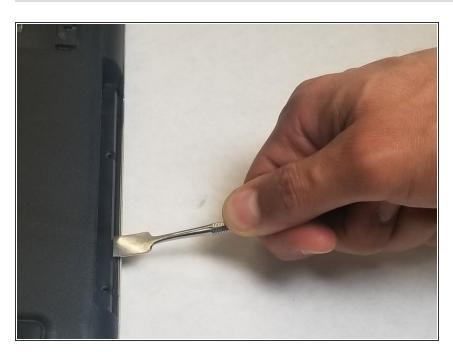
Use a metal spudger to dislodge the optical drive from the connector.
