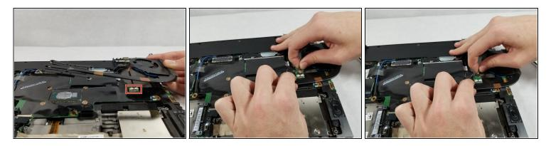
• Lift the fan out of it's compartment to gain access to the cable connection, firmly grab the cable and pull it out of it's housing.
