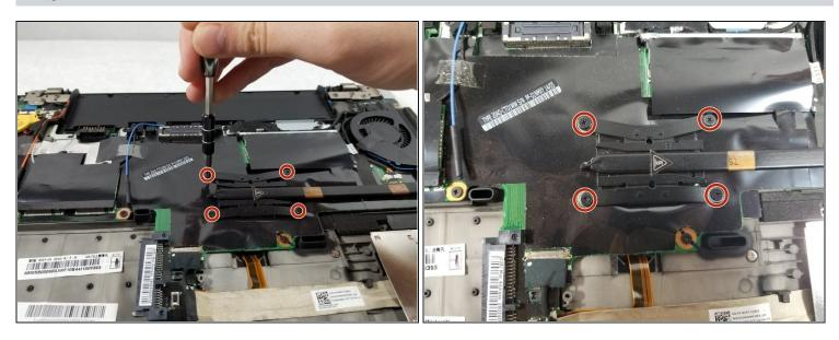
• Use the Phillips #1 screwdriver to remove the four screws holding in the fan assembly.
