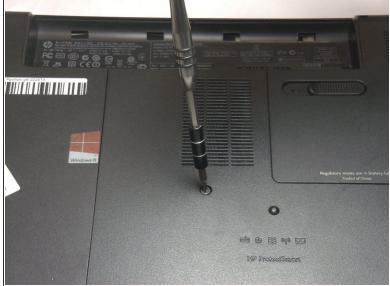
• Use a Phillips #0 screw driver to loosen the screw. The screw will not detach from the cover.
