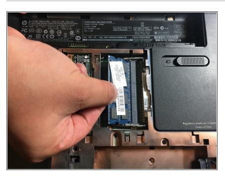
Pull the RAM stick to the left and remove it from the device. To reassemble your device, follow these instructions in reverse order.
