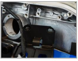
Remove the screws from the battery cover using a Philips #1 screwdriver.
