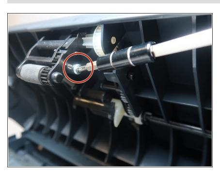
Remove the 10mm screw on the side of the roller with T8 torx security screwdriver.
