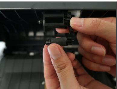
Pull the side cover of the paper-feed roller to the right and remove the paper roller.
