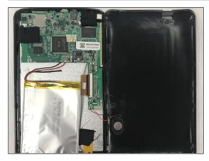
Remove the cover from the back of the tablet. Using the pick tool, pry the cover the case. Do this by starting in the upper corner, working around the edges until the cover unclips from the case.
