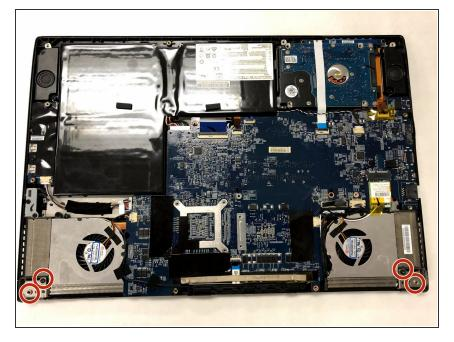
Remove the four 2.5mm screws using a Phillips #1 bit.
