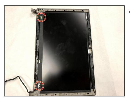
Remove two 2.5mm screws with a Phillips #1 screwdriver.
