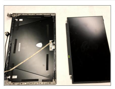
The defective screen is now completely removed and ready to be replaced.
