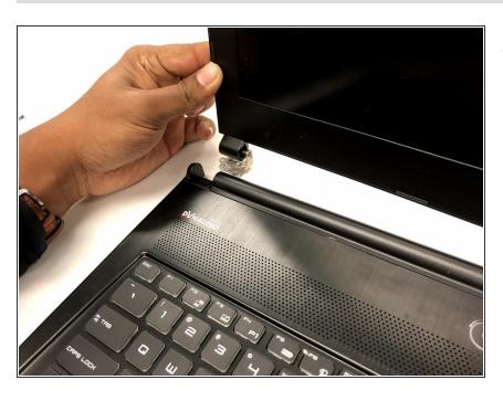
Carefully pry the screen assembly from the chassis on both sides. Use caution as the cable to the screen is located on the right bracket.
