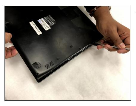
Remove the bottom plate from the laptop. Using a prying tool to slide between the bottom plate and chassis will result in easier removal.
