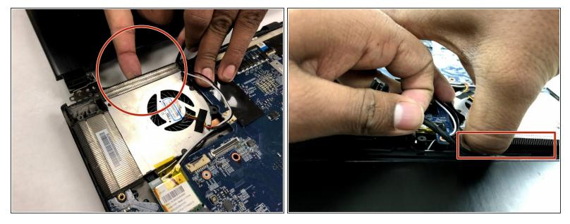
Gently lift up on the back of the fan and remove the routed cable.
