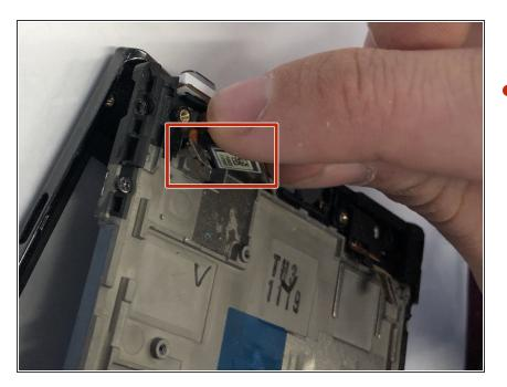
Carefully pull the ribbon cable upward and away from the front screen display.
