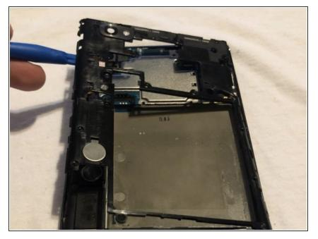
Carefully use the plastic opening tool to pry the plastic shield from the motherboard. This will expose the motherboard and ribbon cables for each component.
