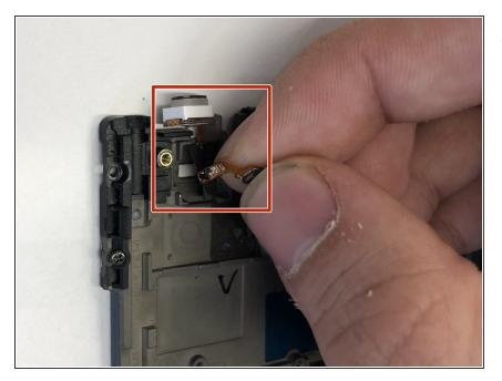
Slowly separate the power button from the screen display. This will release the power button.
