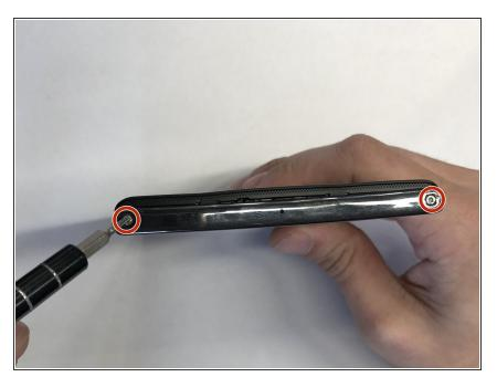
Remove the two 7mm screws holding the back panel of the phone using the P5 bit and magnetic driver.
