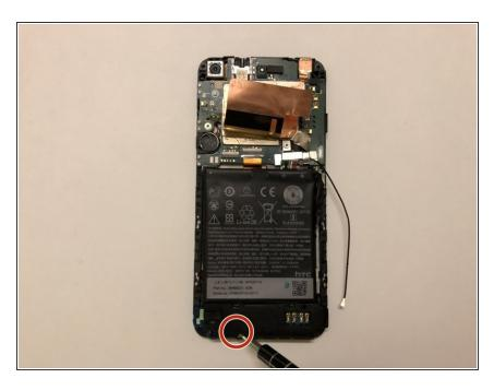
Use the screwdriver to remove the 1.2 mm screw at the bottom of the phone.
