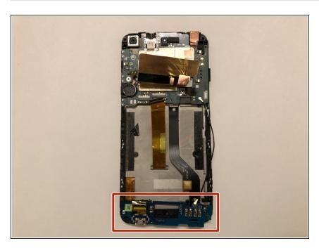
Once the screw and the black plastic backing are removed the daughterboard pulls right out.
