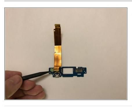
In order to fix the Micro USB Port, the entire daughterboard will need to be replaced because all connections are soldered in.
