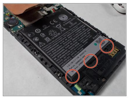
Gently pry the battery up at these three spots, and disconnect the power cables attached.
