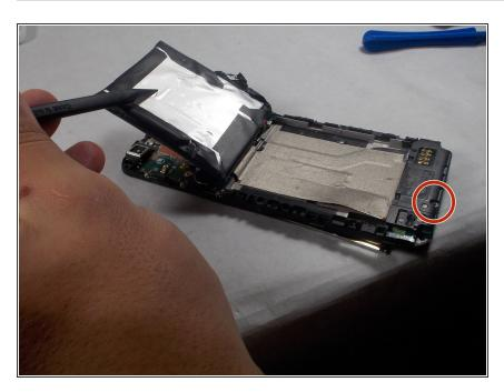
You can then fold the battery back like so, and that will give you access to the screw.
