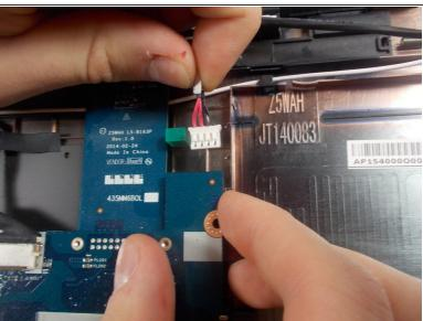
• Disconnect the opposite end of the power jack from the motherboard by carefully pulling the wire.
