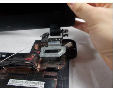
Lift the bottom right side of the screen to move the metal plate covering the power jack.
