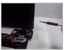
Remove the marked screws with the JIS #00 screwdriver.
