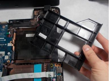
Remove the plastic safeguard from the CD drive slot.
