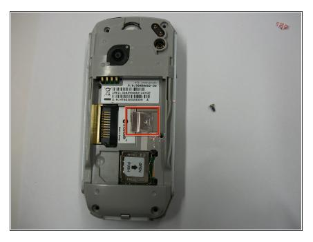
Secure the SD card in place by sliding the silver tab over it (SD card not pictured).
