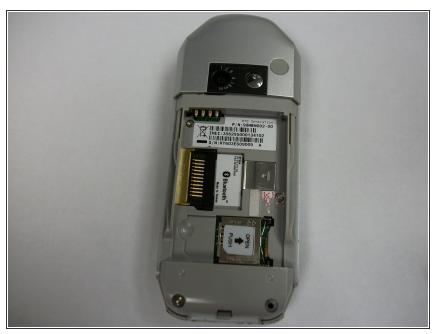
Locate the slot for the SD card on the back of the phone. Insert the SD card so that the copper connectors on the card line up with the connectors on the phone (no card pictured).
