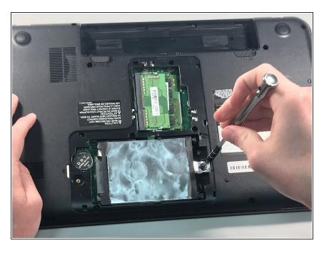
Using the Phillips #1 screwdriver, remove the 8mm screw that is holding the hard drive in place.
