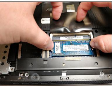
Lift up the plastic static shield atop the RAM slots.
