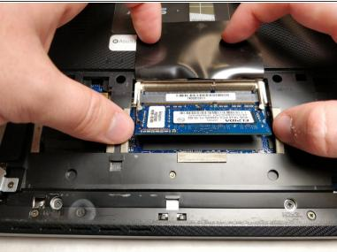
Depress the tongs on either side of the RAM stick to loosen the RAM from the slot.
