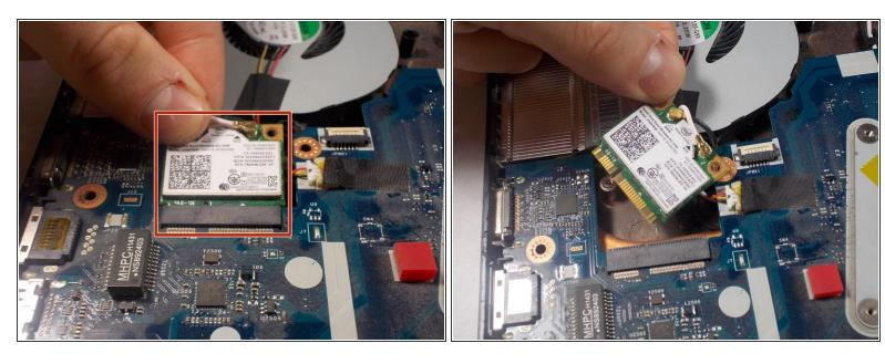
Carefully pull the marked green chip out of the motherboard.
