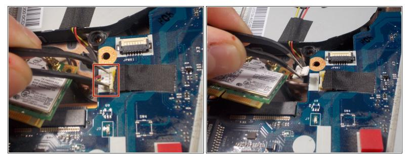
Use tweezers to unplug the wire connecting the fan to the motherboard.
