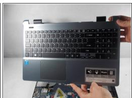
Remove the top panel of the laptop with the plastic opening tool.
