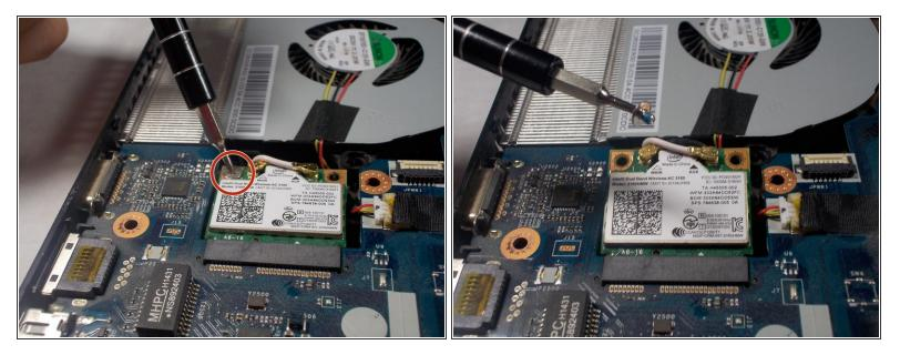
Use a JIS #000 screw bit to remove the marked screw.
