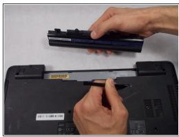
• While the battery release switch is pushed to the right, carefully slide the battery out of its socket.
