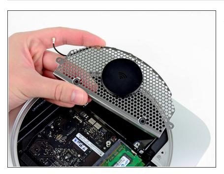
Remove the antenna plate from the mini.
