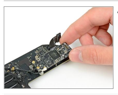
Remove the AirPort/Bluetooth board from the logic board.
