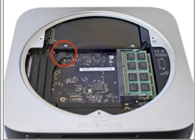
Use the flat end of a spudger to pry the hard drive connector up from its socket on the logic board.
