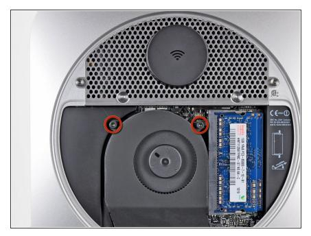
Remove the two 11.3 mm T6 Torx screws securing the fan to the logic board near the antenna plate.
