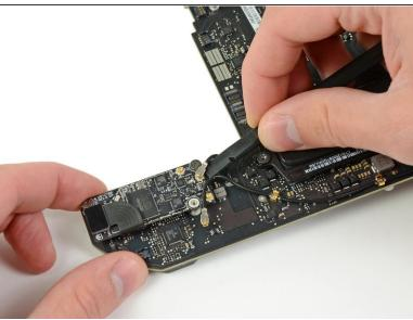
Use the flat end of a spudger to pry both antenna connectors up from their sockets on the AirPort/Bluetooth board.
