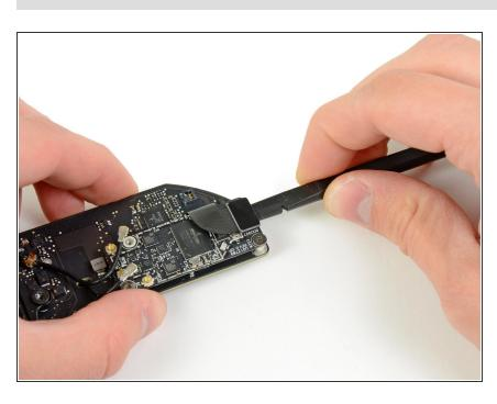
Use your spudger to help disconnect the AirPort/Bluetooth ribbon cable from its socket on the AirPort/Bluetooth board.
