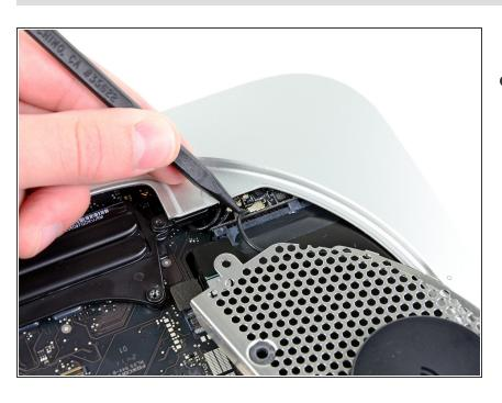
Use the tip of a spudger to carefully pry the antenna connector up from its socket on the AirPort/Bluetooth board.
