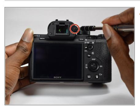
Remove the screw from the middle of the diopter with the JIS #00 screwdriver.
