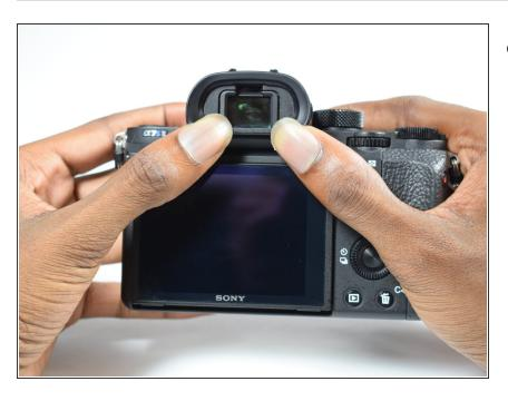
Place each of your thumbs on the interior portions of the eyepiece cup, pressing down and pushing up.
