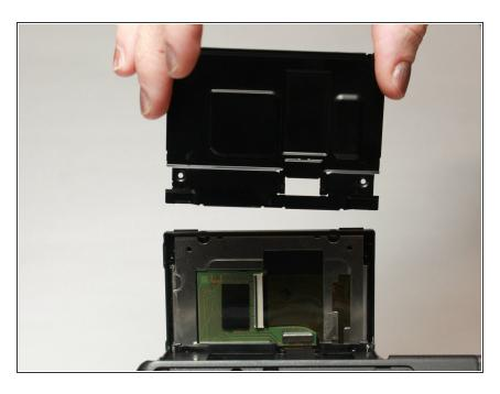
Carefully remove the back of the LCD cover.
