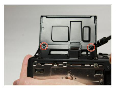
Lift the LCD screen to unscrew the 2 screws on its underside.
