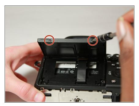
Unscrew the 2 screws on the bottom of the LCD screen.
