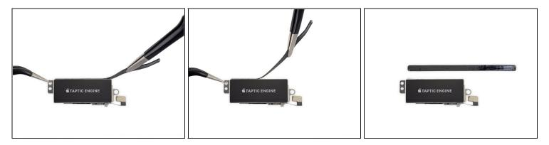
Peel up and remove the plastic bumper strip from the Taptic Engine.
