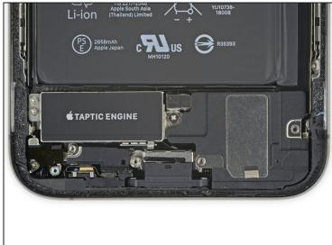
• Remove the 1.9 mm Phillips screw securing the speaker connector cover.
