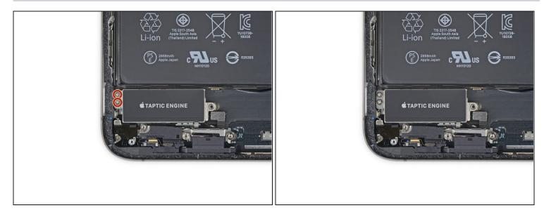
• Remove the two 1.9 mm Phillips screws securing the Taptic Engine.
