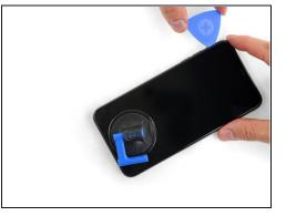
• Slide the opening pick around the lower left corner and up the left edge of the iPhone, slicing through the adhesive holding the display in place.
