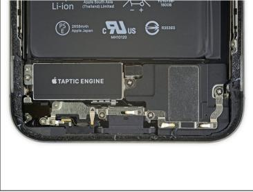
• Remove the five 1.4 mm tri-point Y000 screws securing the bracket below the Taptic Engine and main speaker.
