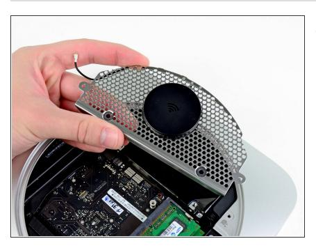
Remove the antenna plate from the mini.
