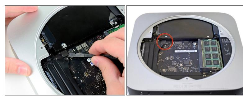
• Use the flat end of a spudger to pry the hard drive connector up from its socket on the logic board.
