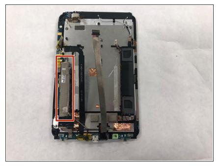
• Remove the camera flex cable.
