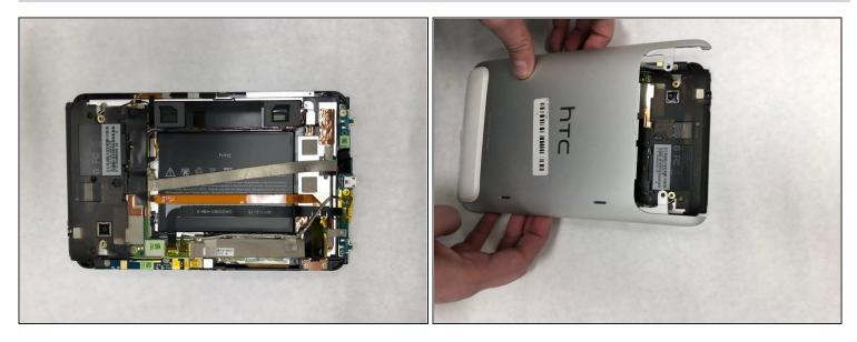
• Remove full frame on the back. A tip is to tape the volume button to the frame before removing it, as the volume button will fall out.
