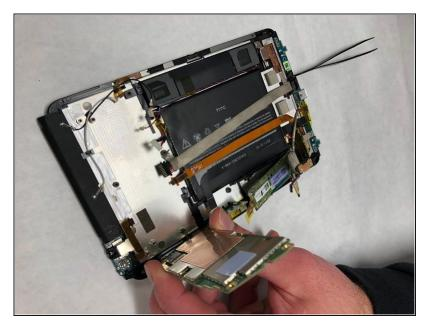
• Release the two file cables attached to the motherboard.
