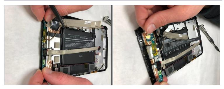
• Remove the dock port flex cable. It will be tangled around other cables, so take care not to rip it while removing.
