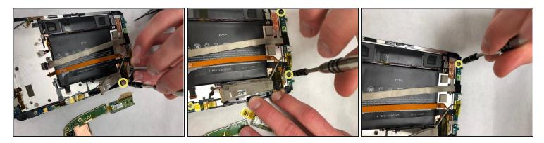
• Remove the motherboard. Note that the flex screen will not be removed with it and will remain attached to the tablet frame.
