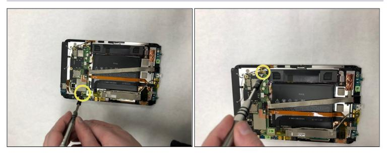
• Remove four T5 Torx screws.
