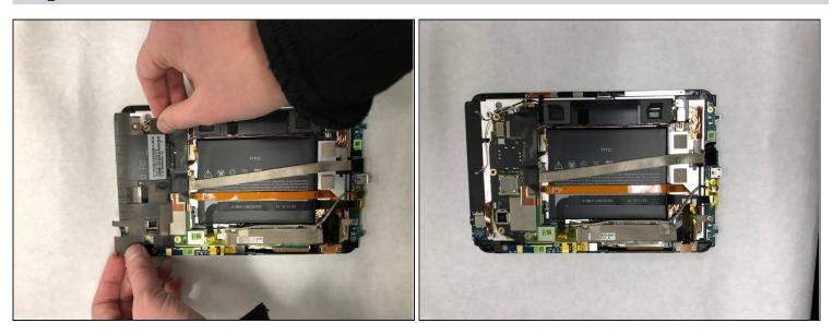
• Remove the plastic top cover of the motherboard.
