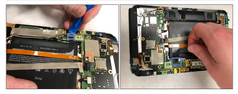
• Release the flex-screen touch cable. It is held in place with clips. Use the safe open pry tool to unclip it. Note that it will still be connected to the base and the motherboard.
