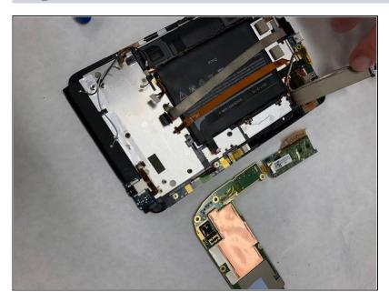
• Remove the motherboard. Note that the flex screen will not be removed with it and will remain attached to the tablet frame.
