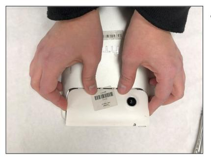
• Remove the white portion of the top cover as shown. Push down on it to slide it off using just your fingers. Be careful not to break the clips holding it in place with removing it.
