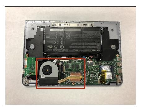
Remove the back cover of the Chromebook and locate the Heat sink and connected fan.
