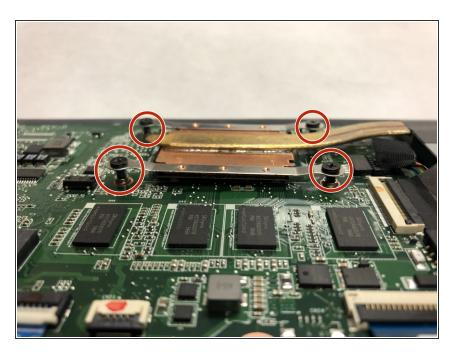
Unscrew the 4 screws connecting the Heat Sink to the motherboard.
