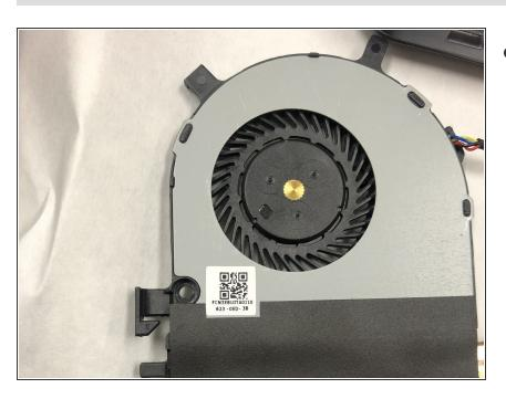
Carefully remove the Heat sink and fan and set aside.
