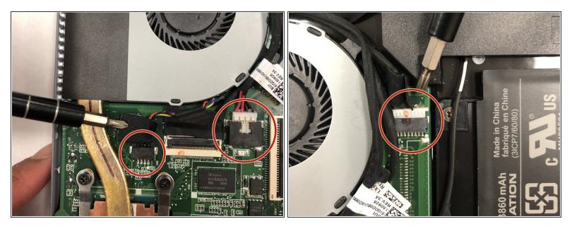
Unplug the three primary wires attached to the fan from the motherboard.
