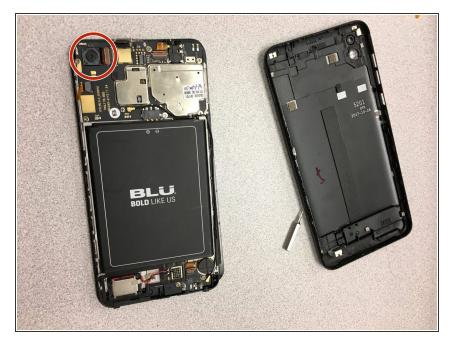
Identify the back-panel camera in the left -hand corner of the open device. (Figure 1)
