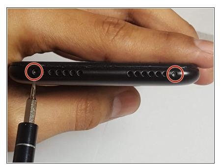
Locate the two torx screws at the bottom of the phone and remove them using the T2 Torx Screwdriver.
