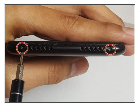
Using a T2 Torx Screwdriver, remove the two screws from the bottom edge of the phone.
