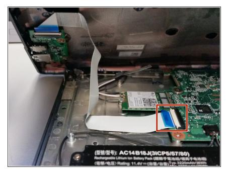
Remove the USB Ribbon cable by opening the connector on the motherboard and sliding the cable out.
