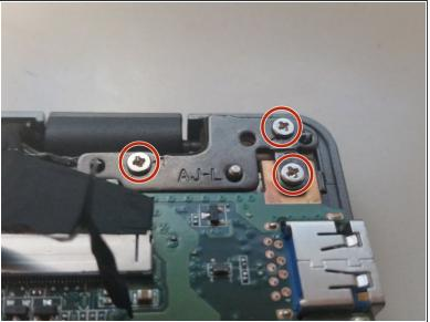
Remove the six screws from the hinges.
