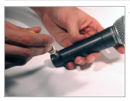
Using a small flat head screw driver, turn the screw in the side of the microphone clockwise until it is tight.
