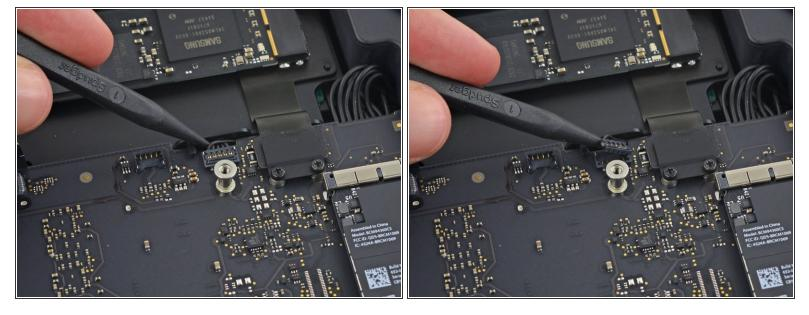
Use the tip of a spudger to disconnect the IR sensor cable connector by prying it straight up from its socket.
