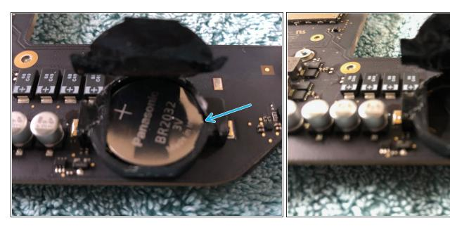
Use a spudger or small screwdriver to push the battery to the side and it will flip out
