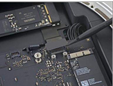
Lift the PCIe SSD connector up off its socket.
