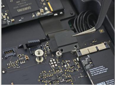
Remove the PCIe SSD cable bracket.
