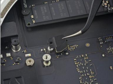
Remove the SATA cable connector bracket.
