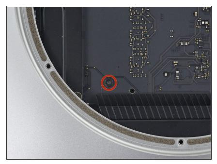
Remove the single 16 mm T6 screw securing the logic board.
