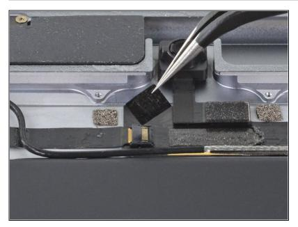
Use a pair of tweezers to remove the sticker covering the left ambient light sensor's ZIF connector.
