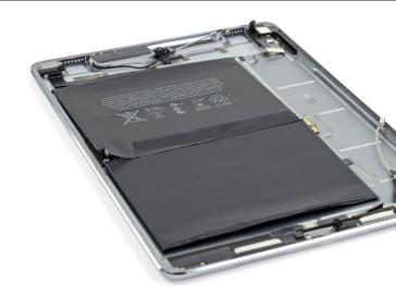
• Place the replacement battery pack so that the two screw posts line up with their holes on the mid-battery circuit board and battery connector.
