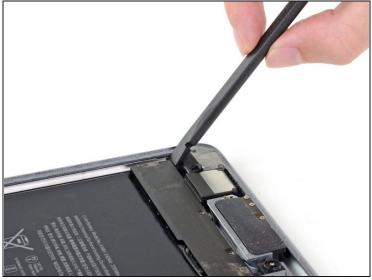
• Use the flat end of a spudger to push the left side of the upper speaker toward the battery just enough for the left speaker to slide out of its recess in the frame.
