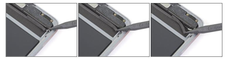
• Use the pointed end of a spudger to detach the foam spacer adhered to the fourth left antenna cable sticker.
