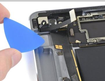
Remove the opening pick from the upper logic board arm.
