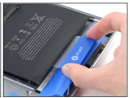
Repeat the application, waiting, and slicing process to release the last adhesive strip located deeper underneath the top battery cell.
