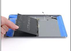
• Use the plastic card or your fingers to flip the bottom half of the battery over so that it rests on top of the upper half.
