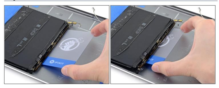
• Slide the long edge of a plastic card about 0.5 inches (13 mm) under the center of the mid-battery circuit board to cut through the remaining adhesive.
