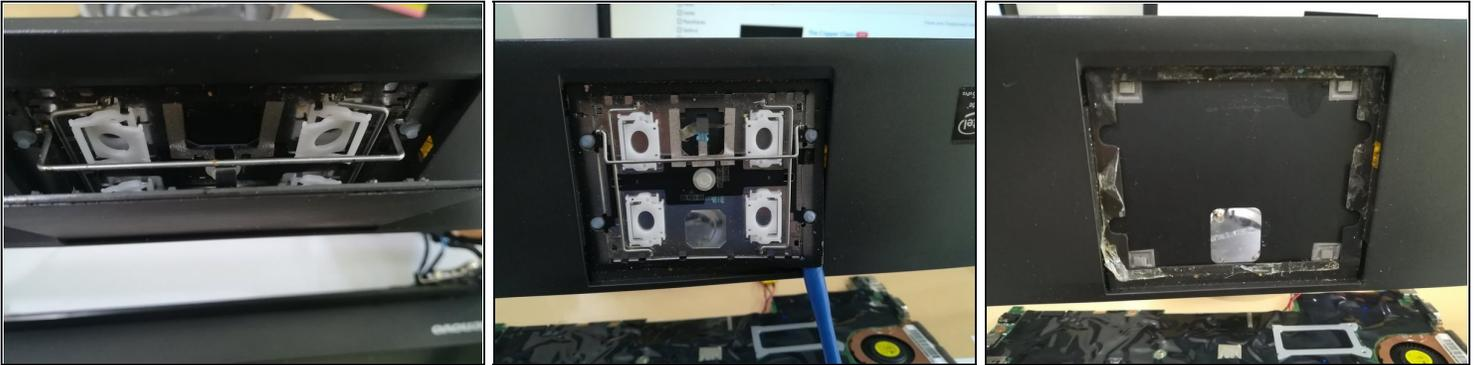
ⓘ As the touchpad is held in place by glue strips, the next steps are necessarily destructive . You should be prepared with a new touchpad that you have confirmed will work before removing the old one.
