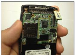
• Use the prying tool to disconnect the rectangular connector.
