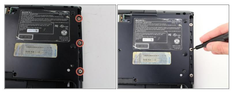
• Remove the three 2mm Phillips #00 screws located on the top right edge.
