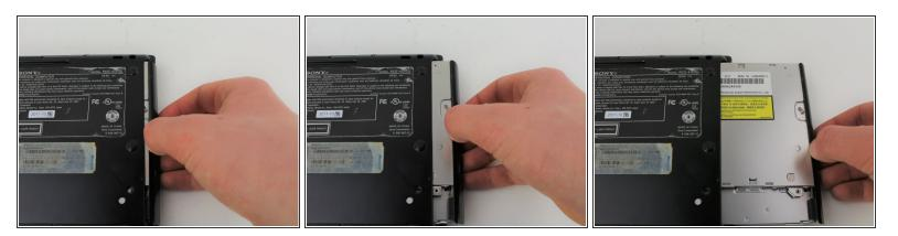
• Carefully remove the disk drive from its compartment.
