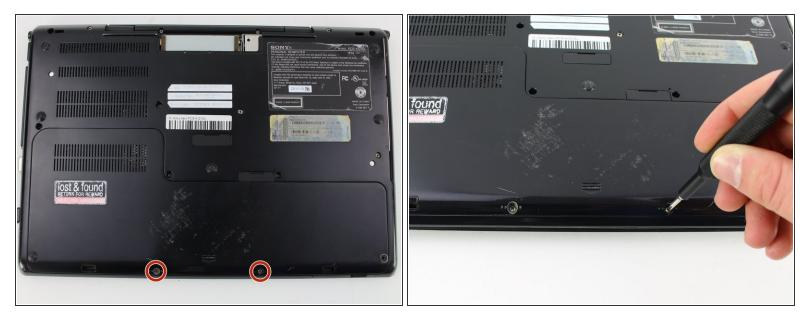
Remove the two 3mm Phillips #0 screws on the bottom of the computer that secure the plastic backing.
