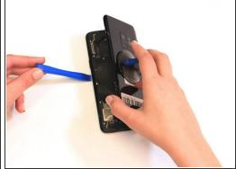
Use the iFixit opening tool to separate the back cover from the rest of the device.
