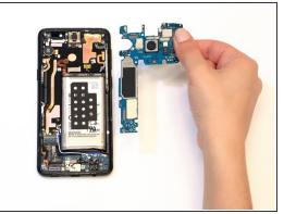
Remove the motherboard by prying it out with the spudger.
