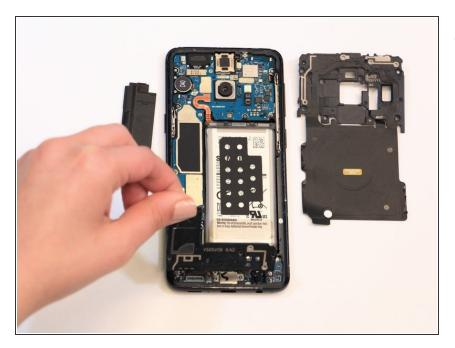
Remove the speaker cover/antenna assembly.
