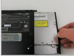
Carefully remove the disk drive from its compartment.
