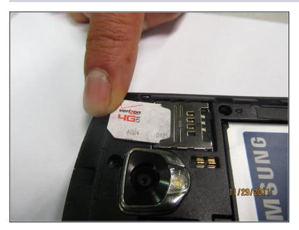
Slide the SIM card out of its casing by pushing on it and sliding it upward.
