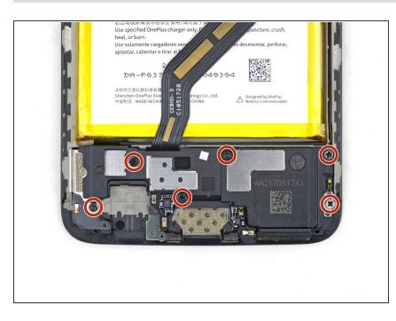
Remove the six 2.6 mm Phillips screws securing the loudspeaker to the frame.
