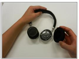
Pull the cushion off of the desired side by gripping the top of the headphones and pulling the cushion off.
