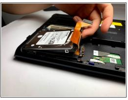
Remove all of the 7mm Phillips #1 casing screws around the hard drive.
