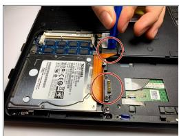
Peel off the ribbon cable, starting at the top by the wifi card.
