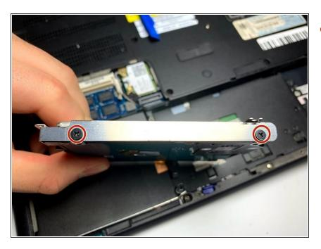
Pull the hard drive out, then remove the 3mm Phillips screws that connect the hard drive to the casing.
