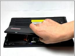
Remove the two 7mm Phillips #1 screws holding the battery cover.
