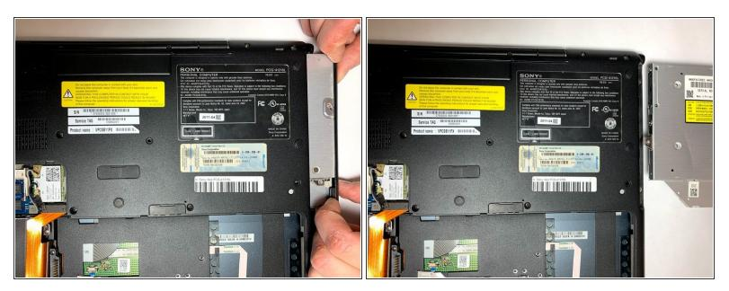
Carefully remove the disk drive by gripping the disk drive by the edges and pulling it out of the computer. Insert the replacement unit in the same orientation and reassemble the unit.
