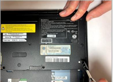
• Remove the two 7mm Phillips #1 screws which hold the disk drive in place.
