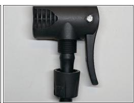
• It's probably easier to work on the head when it is separate from the pump, so unscrew the cover on the hose at the pump head. You may need to use pliers to get enough grip.
