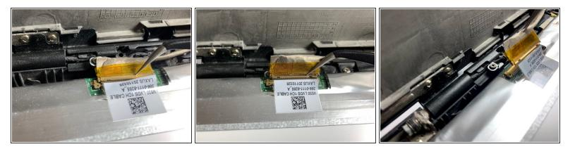
• Use a pair of tweezers to remove the ribbon cable from the screen.
