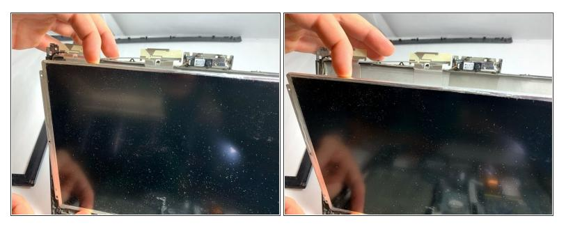
• Carefully remove the screen from the supporting frame and lay it down on the keyboard of the laptop.
