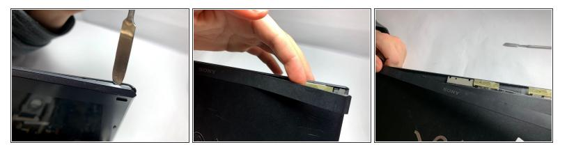
• Use a metal spudger to separate the top cover on the back of the screen. It will be a long, thin plastic section that has the SONY logo in the middle of it. This enables the disassembly of the rest of the screen frame.
