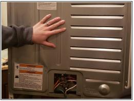
Now that we have safe access to the rear panel we must first remove the small plate on the back of the dryer. To do this simply unscrew the single screw at the top of the small plate and lift the plate out.
